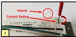
Using a small hex handled flathead screwdriver, gently turn ONLY the screw for the current setting in the clockwise direction, all the way until it stops.
