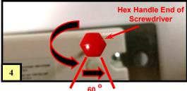
Turning screwdriver one "flat", or approximately 60 degrees, is shown in Figure 4 at left. After both voltage and current screws have been adjusted, replace the inserts back to the power supply (as seen in Figure 1)
