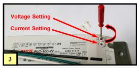
Next, turn BOTH screws to adjust the voltage and current settings in the counterclockwise direction by one "flat", as determined on the hex handle end of the screwdriver (approximately 60 degrees). Refer to Figure 4 below.
