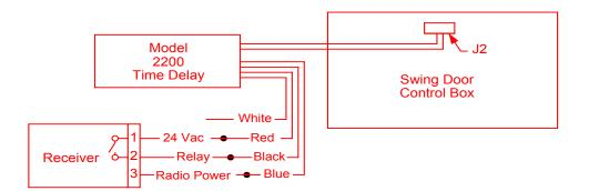
5. Turn the power ON and activate the door. Adjust the potentiometer on the module to achieve the desired time delay. It is adjustable from 1 to 60 seconds.
