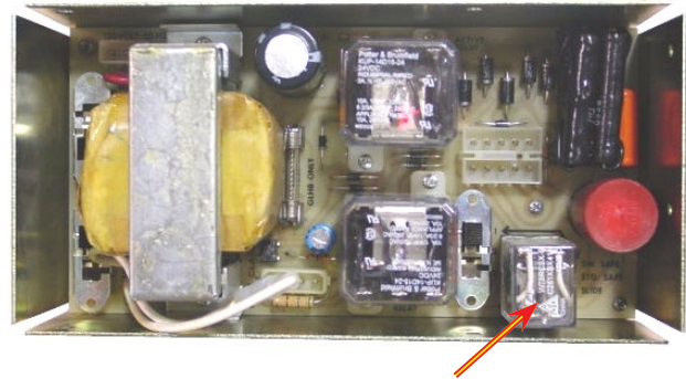
Relay Installed in this Socket
