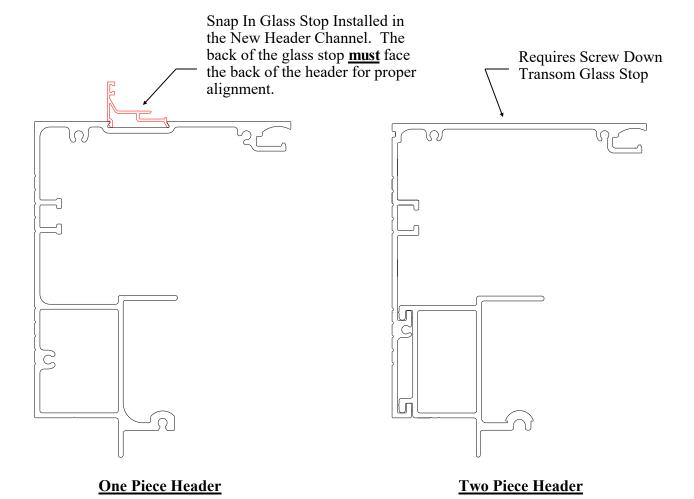
**<u>Benefit</u>**: The new snap channel will save installation time on a unit with transom, no more drilling and screwing down glass stop on the top of the header.
