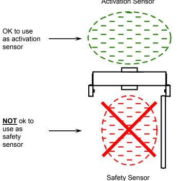
If a swing side safety sensor is required, we recommend the following sensors be used for this purpose:
